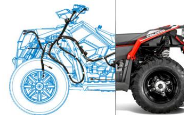
Main Power Harness
